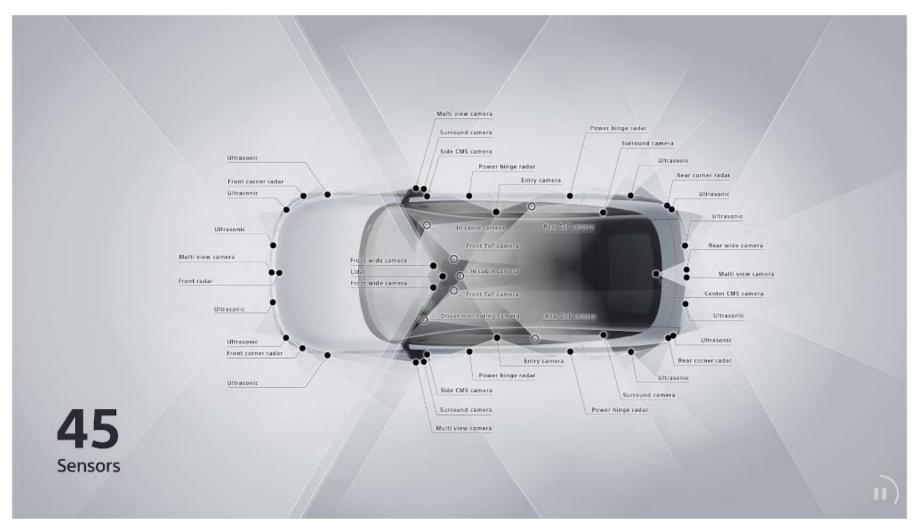
45 sensors are equipped inside and outside the vehicle not only for realizing safety functions but also for entertaining passengers
