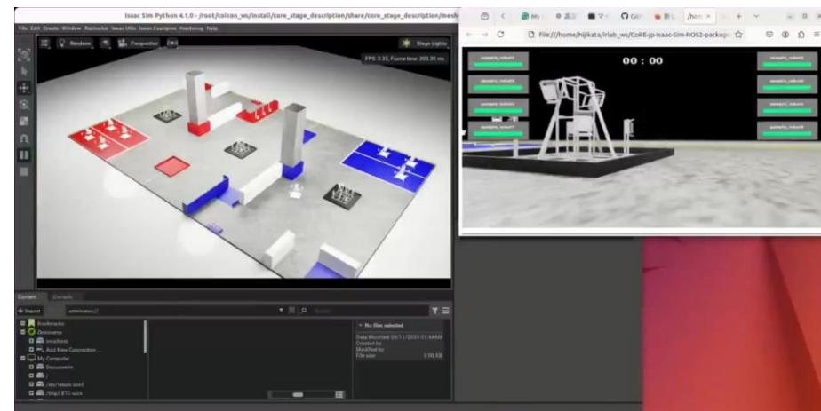
Isaac Sim can run at 10 fps with 4 robots and 80 disks in total.
